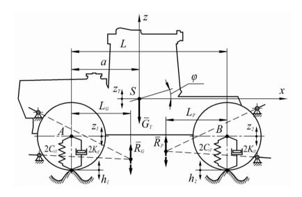
Construction of a mathematical model of the movement of an agricultural machine unit.
